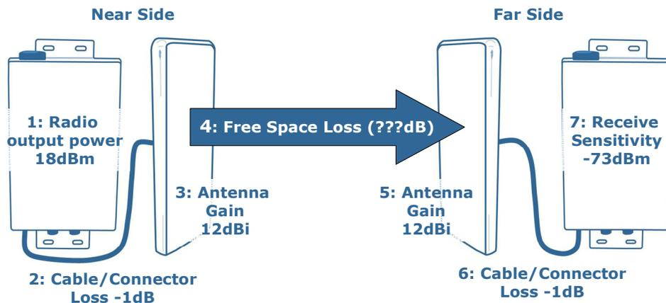
**Figure 5: Radio output power, cable losses and receive sensitivity are known values**
